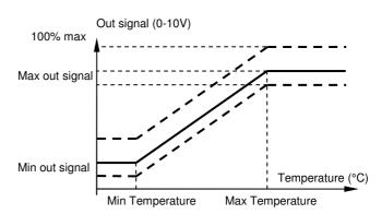
Figure 8. Change of out signal reference.
