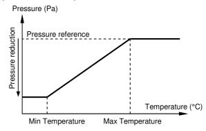
Figure 4. Outside temperature compensation.
