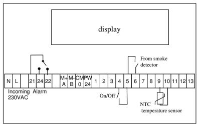
Figure 1. Connection for pressure control with fixed out signal activated by smoke detector. Outside temperature sensor connected on terminal 9, 10.
