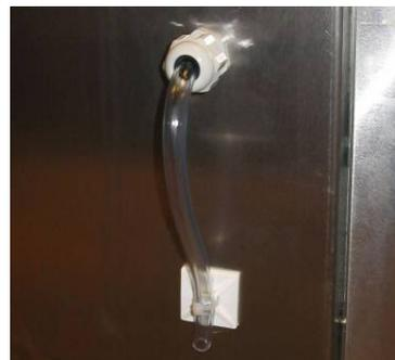
Figure 2. Mounting of pressure hose for measuring of atmospheric pressure.
